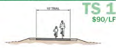
TS 1: Natural Bench/Minor Grading
