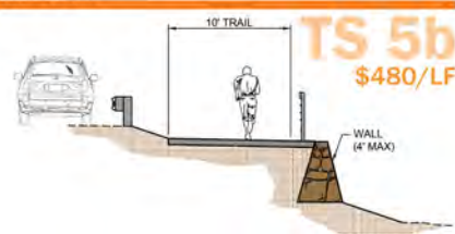
TS 5b: Attached Trail/Minor Fill Walls/Guardrail
