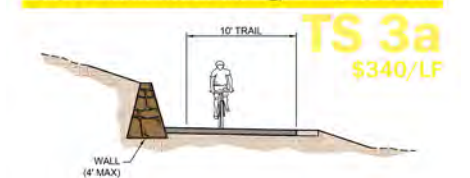
TS 3a: Moderate Grading/Minor Cut Wall
