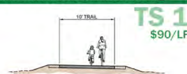
TS 1: Natural Bench/Minor Grading
