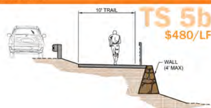
TS 5b: Attached Trail/Minor Fill Walls/Guardrail
