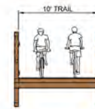
TS 7b: Prefabricated Multi-Span Pedestrian Bridge
