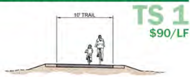
TS 1: Natural Bench/Minor Grading
