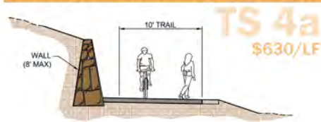
TS 4a: Significant Grading/Major Cut Wall
