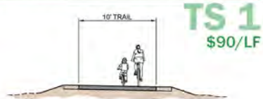
TS 1: Natural Bench/Minor Grading
