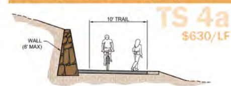
TS 4a: Significant Grading/Major Cut Wall
